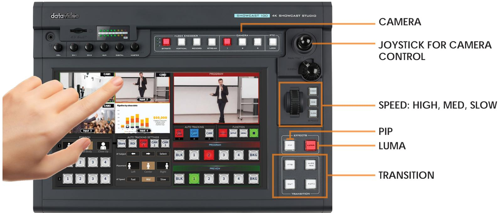
The Showcast 100 is an unique 4K, 4-input switcher with tactile buttons, joystick camera control and 14" touchscreen with multi-view, program and advanced menu options.
